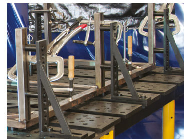
Adjustable fixturing with V-Blocks
